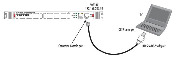
Figure 12. Connecting the 6081RC to your laptop PC via the console port
